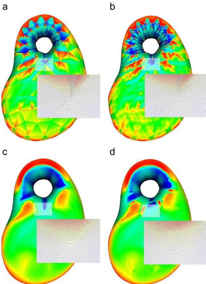
Fig. 10. Curvature plots for the surfaces generated from mesh model 1: (a) PN triangle; (b) PPS from the surface in (a); (c) Loop; and (d) PPS from the surface in (c).
