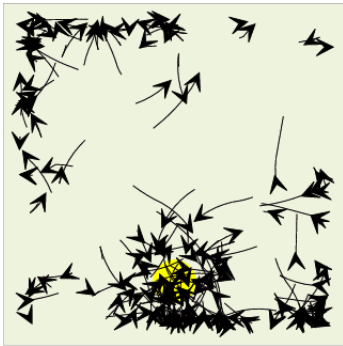
Fig. 4. The endStates (depicted as arrow heads) of all 169 goals found in one run. The paths the robot took during the 10 actions before reaching each endState are also shown as black lines attached to each arrow head.
