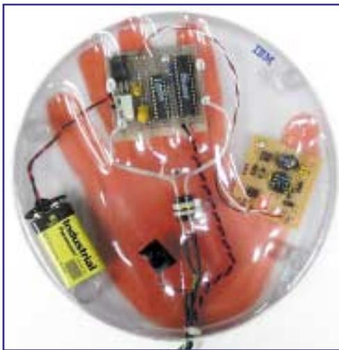
IBM's Emotion Mouse II was designed for correlating pulse, temperature, general somatic activity, to galvanic skin responses. By using this mouse, you can provide additional input to a system.
