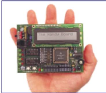
The Handy Board, by MIT's Fred Martin, is an open architecture with complete specs for building, and code for running, on their web site.
