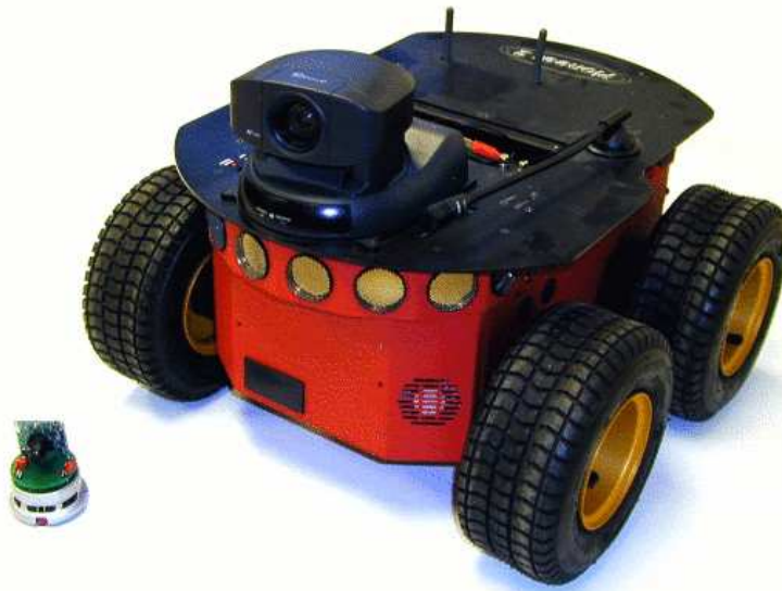
Figure 3: Two very different robot platforms, the tiny Khepera and the much larger Pioneer, for which the same Pyro program from Figure 2 can be used for wall following.
