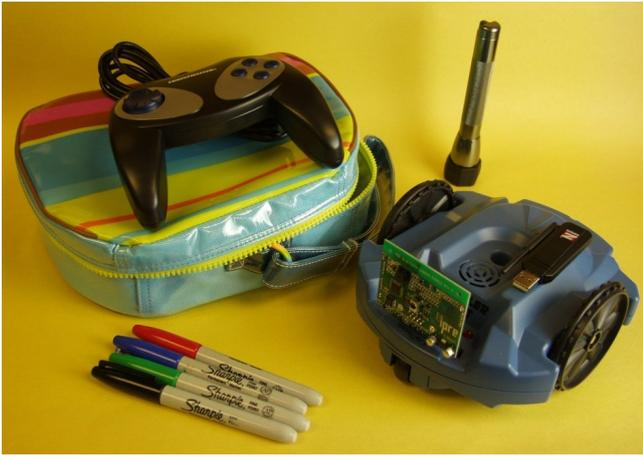
**Figure 1: The IPRE Robot Kit, Fall 2007.** Clockwise, from top-left: lunchbox carrying case, gamepad, flashlight, Scribbler robot with IPRE Fluke (camera and serial Bluetooth adaptor), USB Bluetooth dongle (for computer if it doesn't have Bluetooth), and drawing pens.
