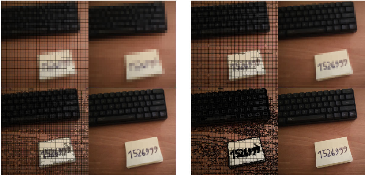
Figure 6: Quadtree image compression, different thresholds
