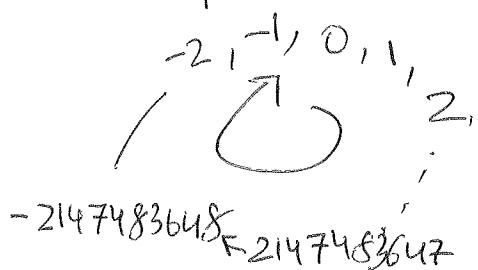
That is when  $i = 2147483647$  is incremented, it results in  $i = -2147483648$ .  $\therefore i$  will again be  $\leq 2147483647$  and so on. It will be an infinite loop !!
