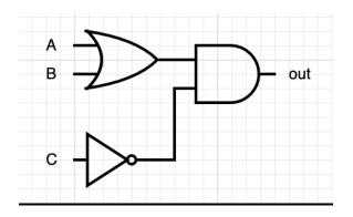
For what inputs does this circuit produce the incorrect output?
