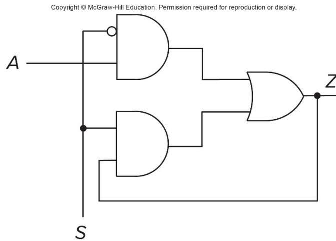
**(a)** What is the output of this circuit at Z when the select line S is 0?
