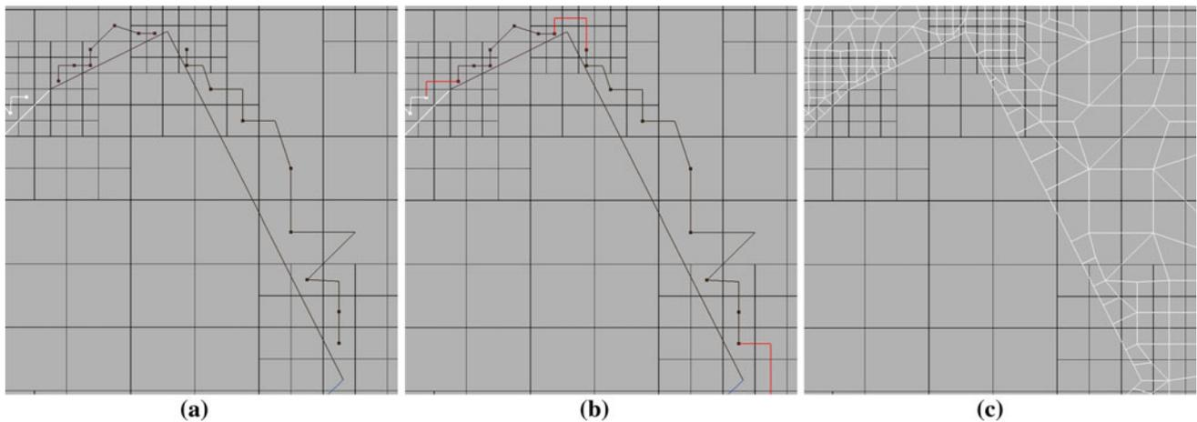
**Fig. 42** **a** Quadrangulation chains for some polygon edges. **b** Connections around corners. **c** Using quadrangulation chains to incorporate edges into  $\mathcal{Q}$
