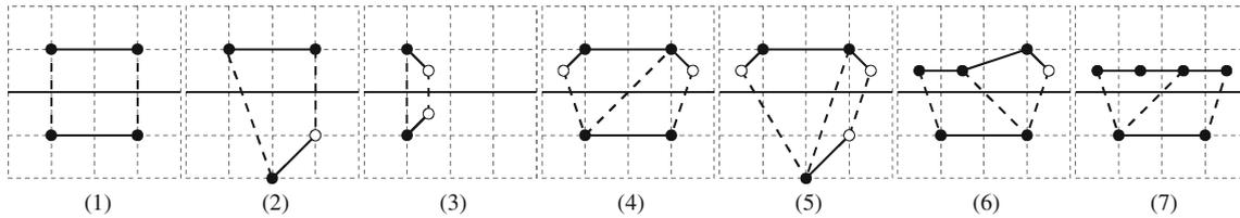
Fig. 5 Stitching 2-2 and 2-4 or 4-2 connector chains
