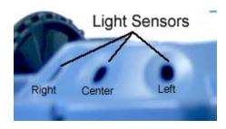
The values being reported by these sensors can be in the range [0..5000] where low values imply bright light and high values imply darkness. The above values were taken in ambient light with one finger completely covering the center sensor. Thus, the darker it is, the higher the value reported. In a way, you could even call it a darkness sensor. Later, we will see how we can easily transform these values in many different ways to affect robot behaviors.
